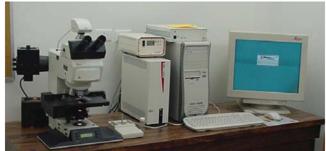
Figure 4. Leica microscope model DMRXA2 equipped with a RGB color 3.2 mega pixel digital camera (Leica model DC300) attached to a 2.5 GHz PC Pentium IV.
